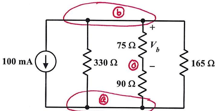
Use the nodal analysis method to determine the value of  $V_b$ .
